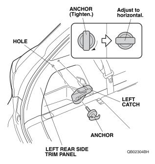
7. Repeat steps 2 through 6 to install an anchor on the right side of the vehicle.
